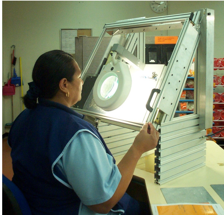
Figure 17. Modified dark fibre detector for AWTA benzyl test method
